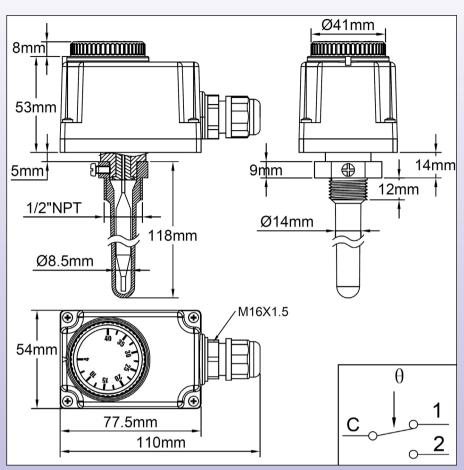
**Housing:** IP44, 77,5 x 54 x 53mm, (Knob and cable gland not included), black PC-ABS, UL94V0. High impact and UV resistance. Stainless steel wall mounting plate, with 2 plastic. **Electrical input:** M16 cable gland.
